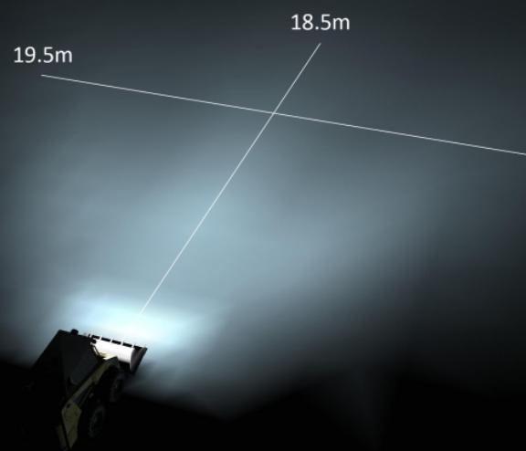
Beam Measurements - 1 Lux
