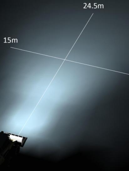
Beam Measurements - 1 Lux
