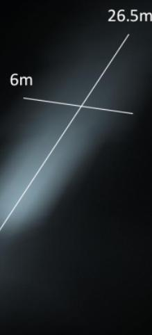
Beam Measurements - 1 Lux
