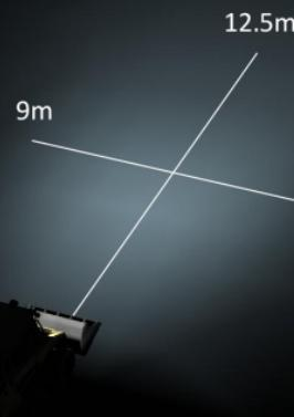
Beam Measurements - 1 Lux
