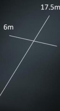
Beam Measurements - 1 Lux
