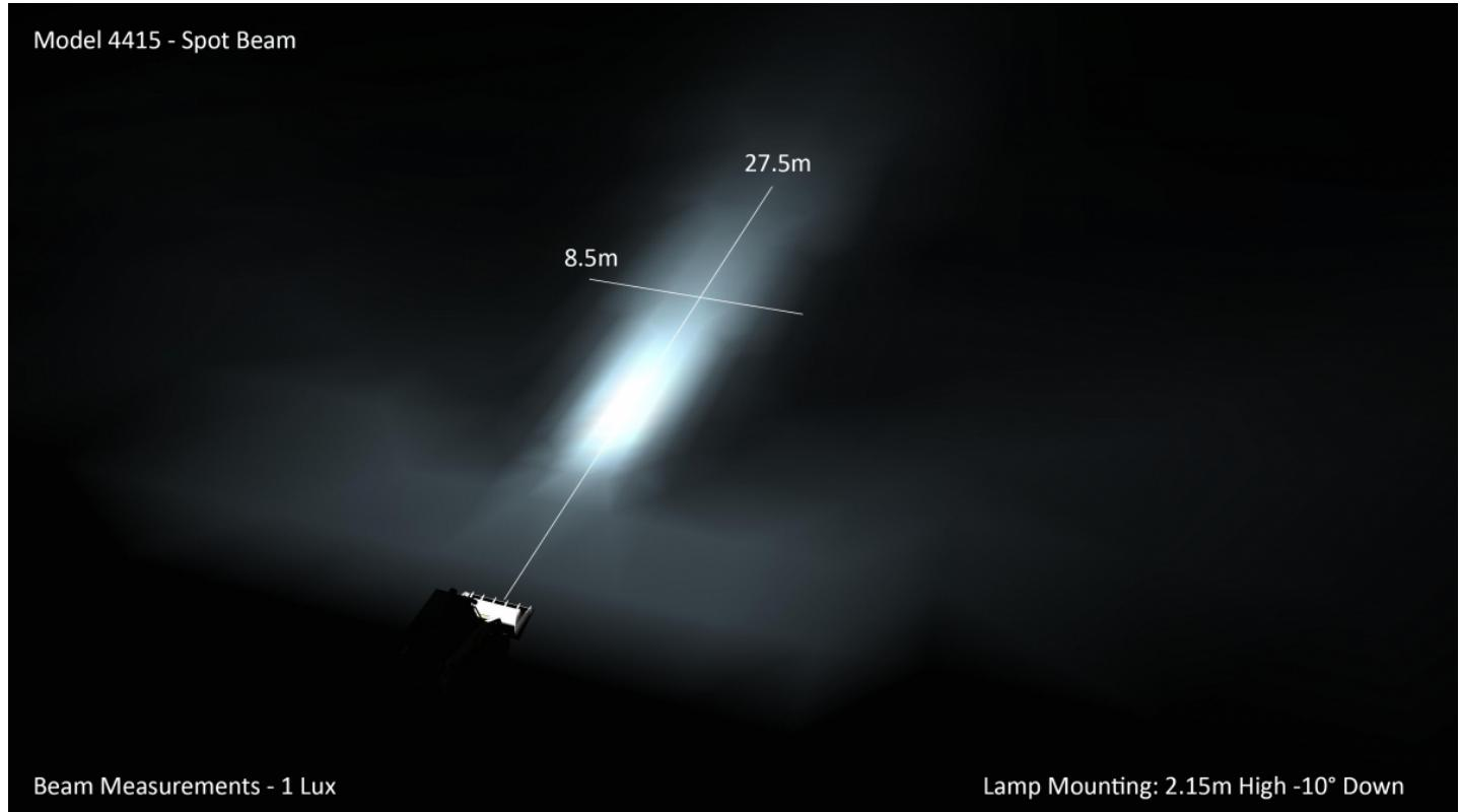
Beam Measurements - 1 Lux
