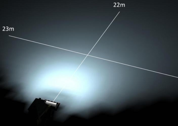
Beam Measurements - 1 Lux
