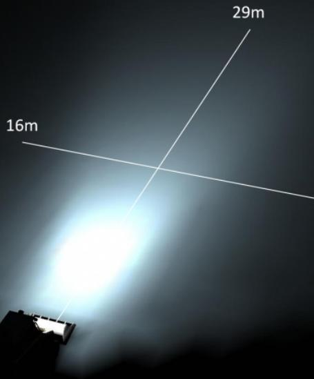
Beam Measurements - 1 Lux
